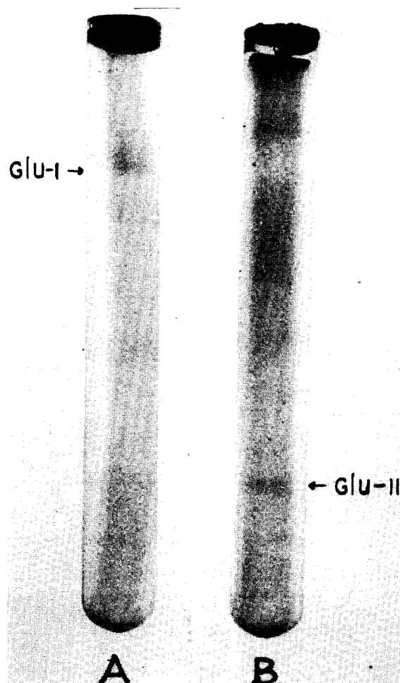
Fig. 2. Cellulose DE-52 column chromatography of (A) \beta -glucosidase I and (B) \beta -glucosidase II obtained from two different pooled fractions from the Sephadex G-100 column.
